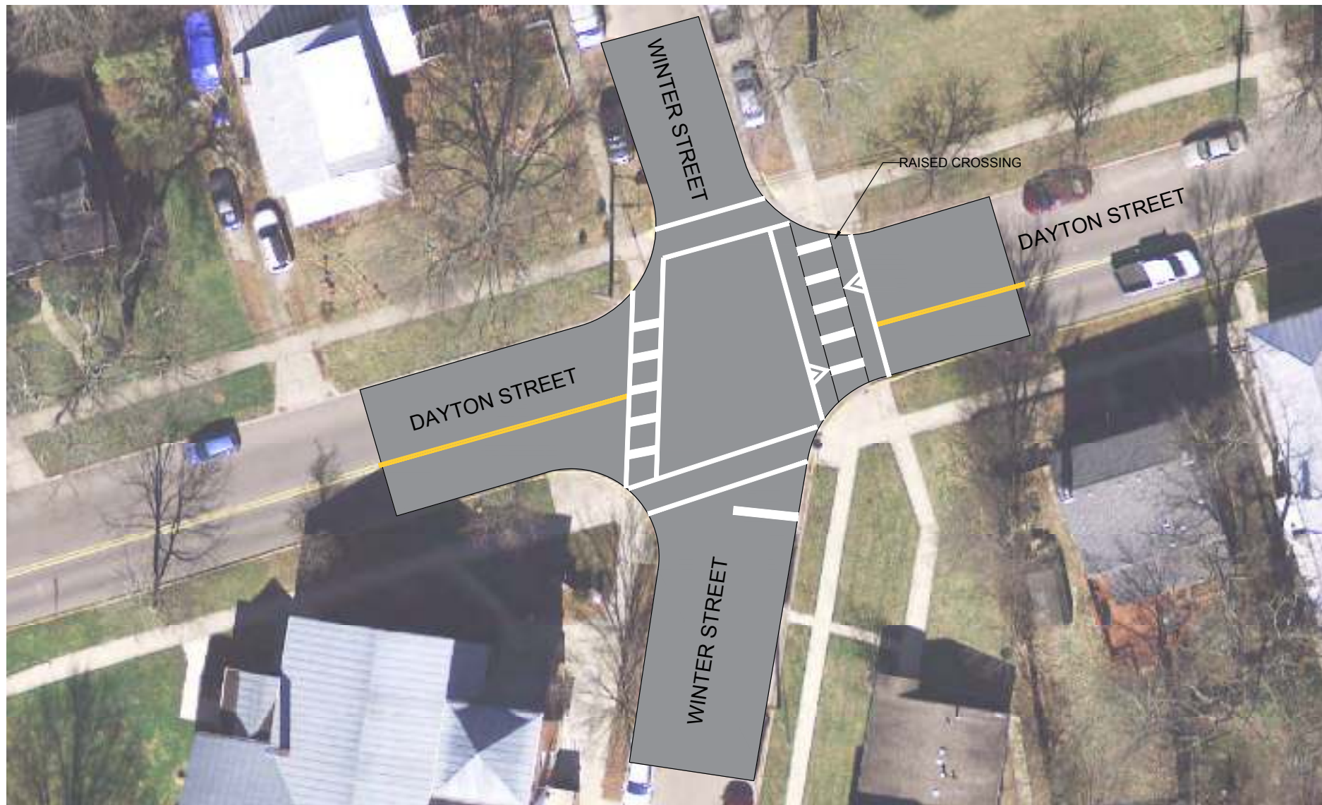
Figure 15: Dayton Street and Winter Street Traffic Calming and Crossing Treatments (S-6)
